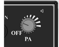
**PA Volume Control** - This knob also provides you the ability to adjust the public address volume. It should be set when the vehicle is parked. Typically you should set the PA volume to the maximum possible level with no feedback (squeal).
